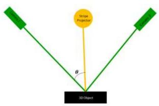
Fig. 3 Structured Light 3D Scanning
