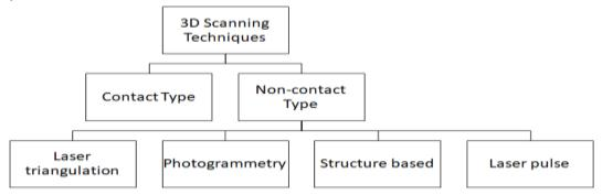
Fig. 1 Classification of 3D Scanning Techniques
