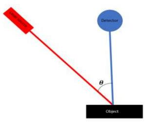
Fig. 2 Laser Triangulation Technique
